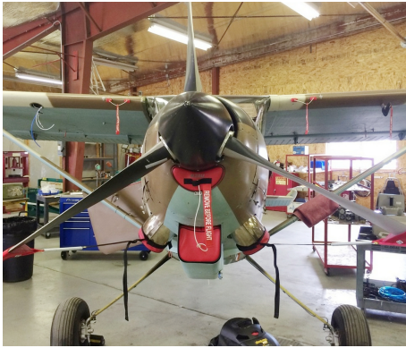
Siai Marchetti 1019 Engine Plugs, Prop Tie-Exhaust Covers
