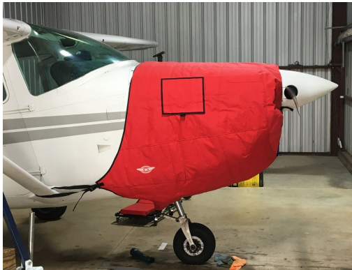
Cessna R182 Insulated Engine Cover, fully enclosed
