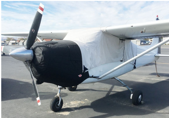
Cessna 182B Insulated Engine Cover, Over-Top Canopy Cover
