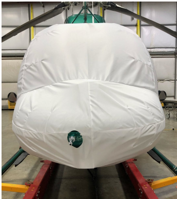
Bell 407 Abbreviated Bubble Cover, secures to doors, test fit cover
