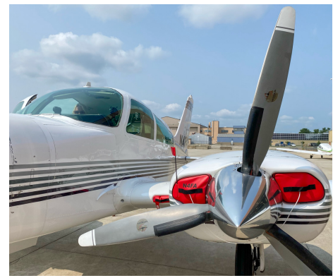
Cessna 310R Engine Inlet Plugs (set of 4)
