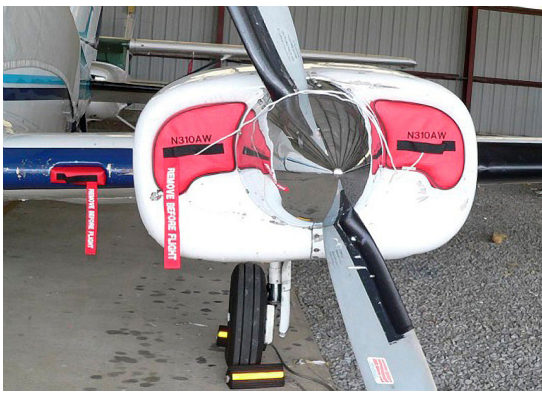
Cessna 310P Engine Inlet and Center Section Inlet Plugs
