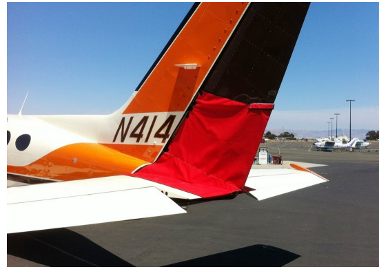
Cessna 414 Rudder Openings Cover (bird barrier)
