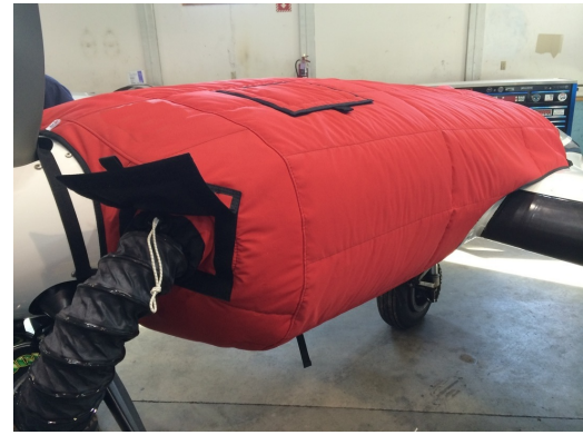
Cessna 402 Insulated Engine Cover with Heater
