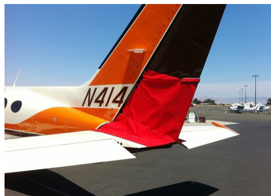
Cessna 414 Rudder Openings Cover (bird barrier)
