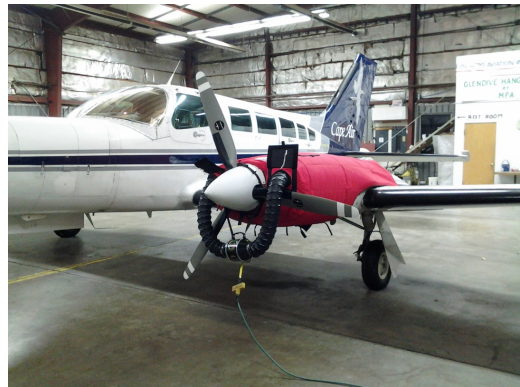
Cessna 402 Insulated Engine Cover with Heater
