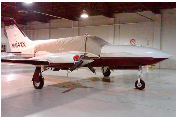
Cessna 414 Canopy Cover and Engine Inlet Plugs
