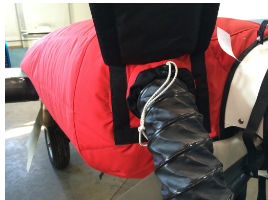
Cessna 402 Insulated Engine Cover with Heater
