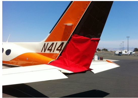
Cessna 414 Rudder Openings Cover (bird barrier)
