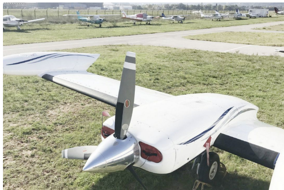
Cessna 340 Engine Inlet Plugs
