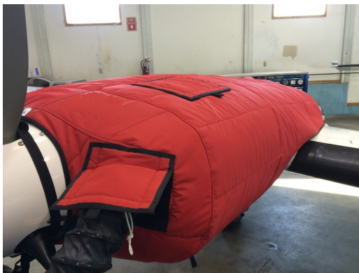
Cessna 402 Insulated Engine Cover with Heater
