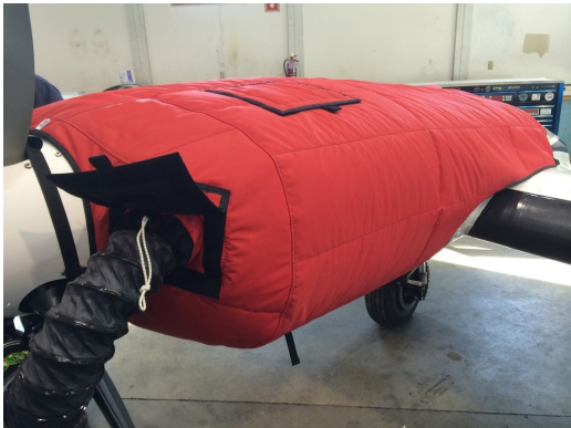
Cessna 402 Insulated Engine Cover with Heater
