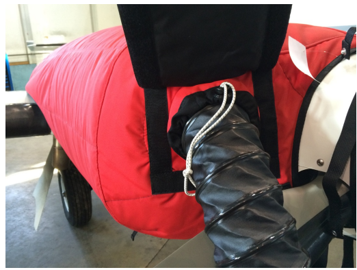
Cessna 402 Insulated Engine Cover with Heater
