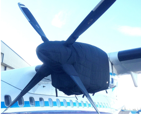
ATR-72-202 Insulated Engine & Prop Hub Covers
