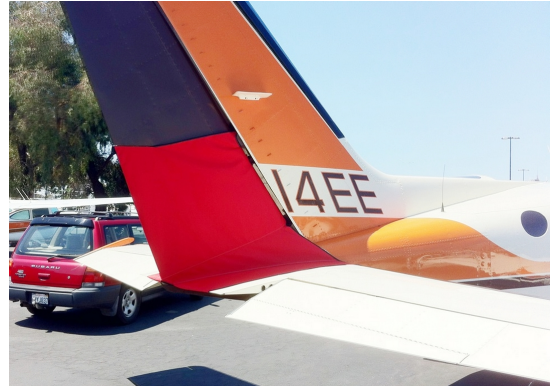
Cessna 414 Rudder Openings Cover (bird barrier)
