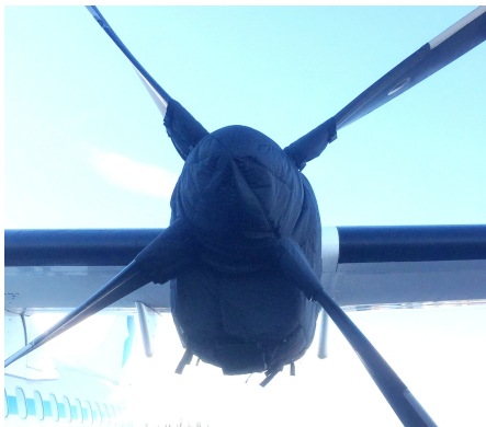
ATR-72-202 Insulated Engine & Prop Hub Covers Prop Tie-Down, Various Models (secures with a hook to engine nacelle)
