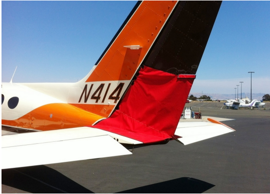
Cessna 414 Rudder Openings Cover (bird barrier)
