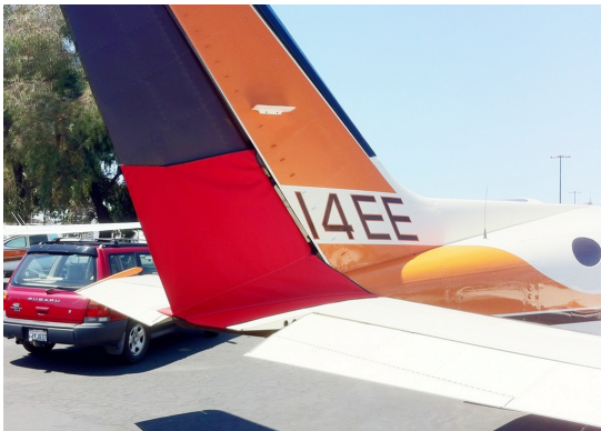
Cessna 414 Rudder Openings Cover (bird barrier)
