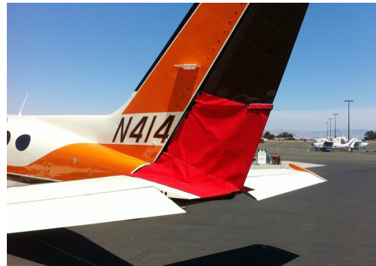
Cessna 414 Rudder Openings Cover (bird barrier)
