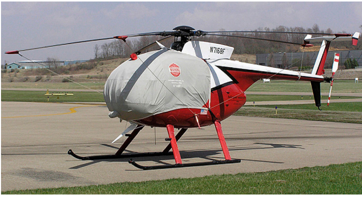
Hughes 500D Bubble Cover with Wire Strike detail and Blade Tie-downs Hughes 500C (369HS) Bubble Cover, Blade Tie-Downs
