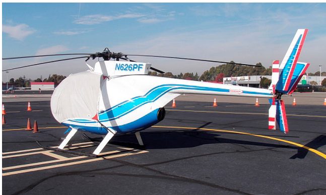
MD500C Bubble Cover with Wire Strike detail
