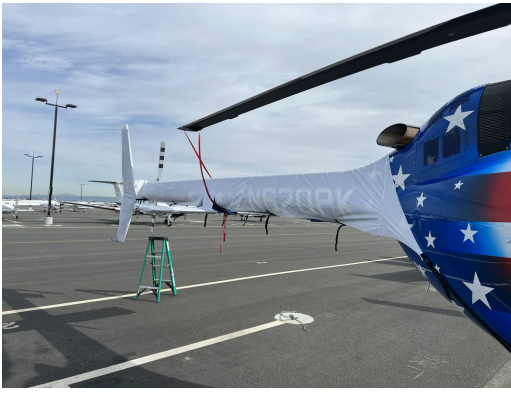
Bell 505 Tailboom & Stabilizer Covers, test fit cover
