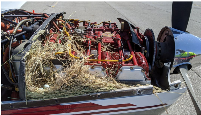
ENGINE PLUGS PREVENT BIRD NEST FOD. Piper Saratoga Engine Cowling Bird's Nest Beech Baron 58P Engine Inlet Plugs
