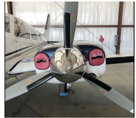
ENGINE PLUGS PREVENT BIRD NEST FOD. Piper Saratoga Engine Cowling Bird's Nest Beech Baron 58P Engine Inlet Plugs
