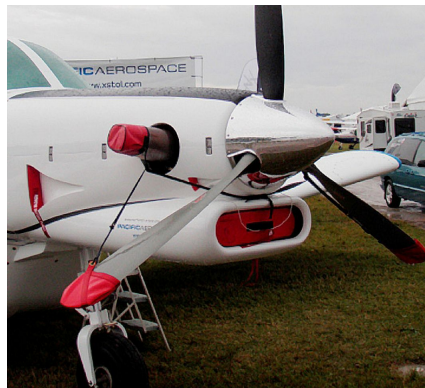
750XL Engine Inlet Plugs & Prop Tie/Exhaust Covers
