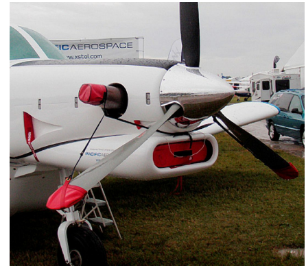
750XL Engine Inlet Plugs & Prop Tie/Exhaust Covers
