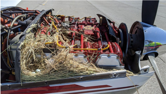
ENGINE PLUGS PREVENT BIRD NEST FOD. Piper Saratoga Engine Cowling Bird's Nest
