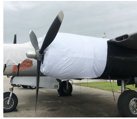
Douglas A-26 Engine Cover, test fit cover
