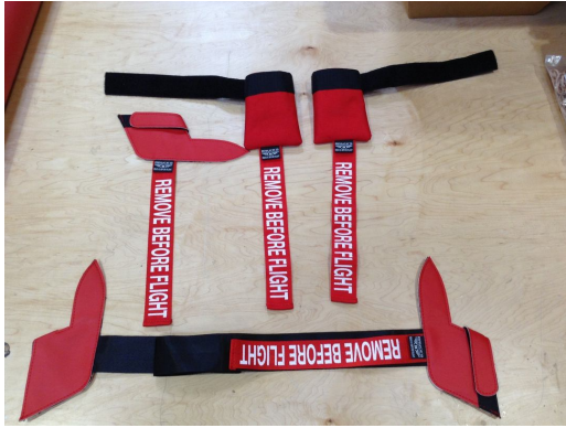
Airbus A319 Pitot & Tat Covers, Heat Resistant Type
