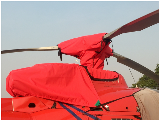
Airbus H-125 & Aerospatiale AS350 Intake/Exhaust Cover, Main Rotor Hub Cover with Weighted Skirt
