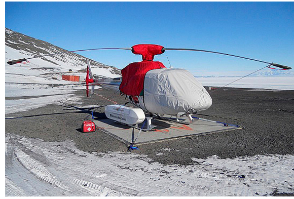
AS350 Bubble Cover w/ Cargo Mirror, Blade Tie-downs, Insulated Engine, Insulated Main Rotor Hub & Insulated Tail Rotor Covers
