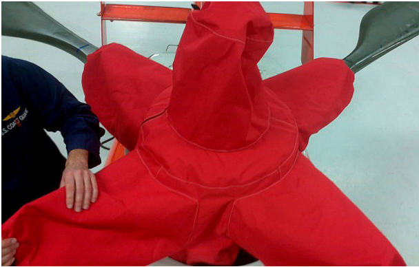
MH-65C Engine Area Cover, Swash Plate Aperture, Rotor Hub cover set, P/N: A365-210 MH-65C Rotor Hub Cover w/ OADS Tube Cover detail
