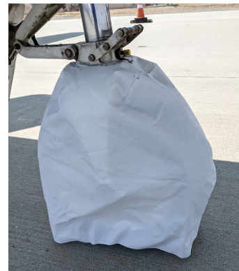
CJ1 Nose Gear Tire Cover, test fit
