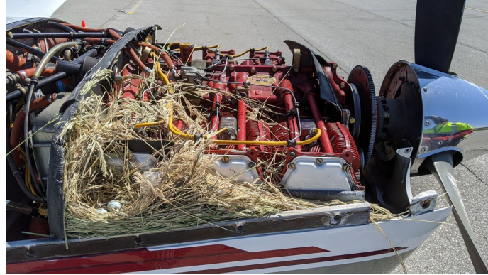
Grumman AA-1A Lynx Engine Inlet Plugs ENGINE PLUGS PREVENT BIRD NEST FOD. Piper Saratoga Engine Cowling Bird's Nest
