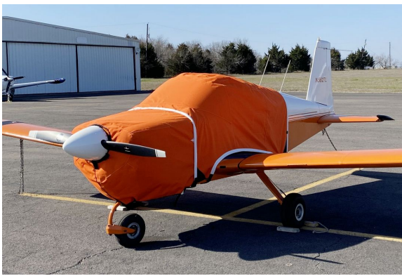
AA-1 Extended Canopy & Fully Enclosed Engine Cover
