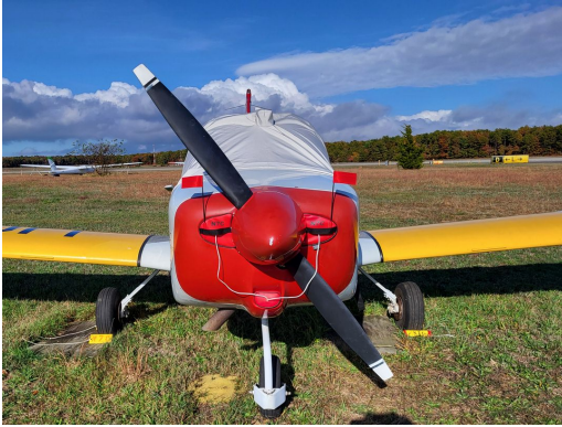
Grumman AA-1A Lynx Engine Inlet Plugs ENGINE PLUGS PREVENT BIRD NEST FOD. Piper Saratoga Engine Cowling Bird's Nest
