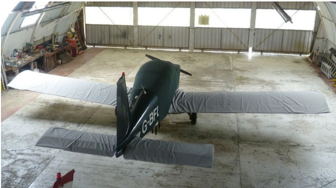
Grumman AA5 Wing & Horizontal Stabilizer Covers
