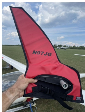
Schempp-Hirth Ventus-2B winglet/wingtip pads
