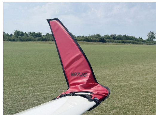
Schempp-Hirth Ventus-2B winglet/wingtip pads
