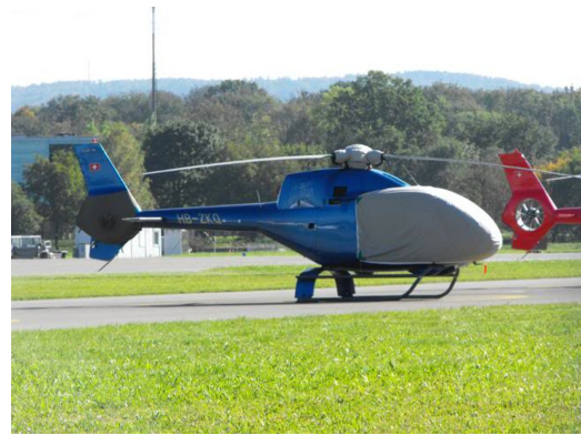
EC-130 Bubble, Tailfan, and Rotor Hub Cover
