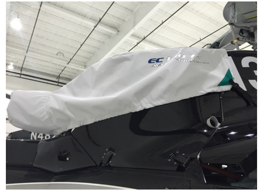
EC-130 Engine Area/Exhaust Cover
