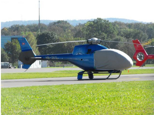
EC-130 Bubble, Tailfan, and Rotor Hub Cover
