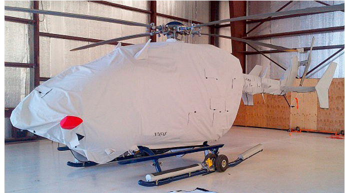
Main Body (also covers bottom), Tailboom, Vertical Pylon, Stabilizers and Tail Rotor Covers
