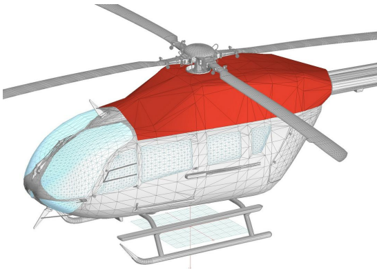
Intake/Exhaust Engine Area Cover, 3D Rendering
