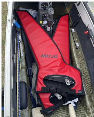
Schempp-Hirth Ventus-2B winglet/wingtip pads
