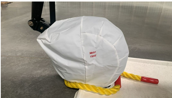
Cub Crafters Tire Covers, tricycle gear, test fit covers
