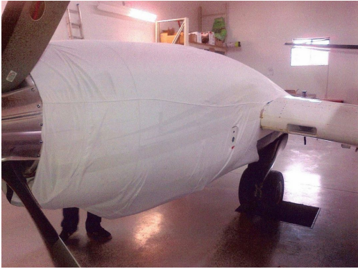
King Air B100 Engine Cover, test fit cover
