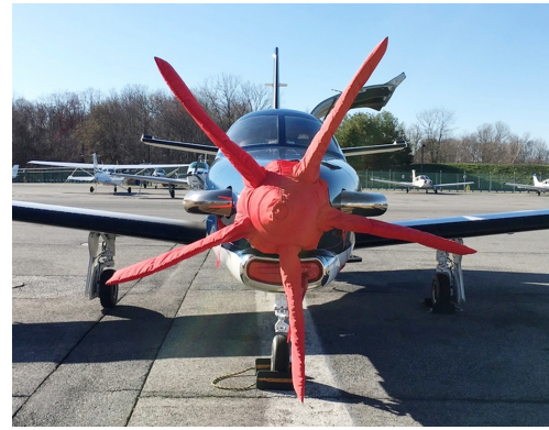
Socata TBM Insulated 5-Blade Prop/Spinner Cover
