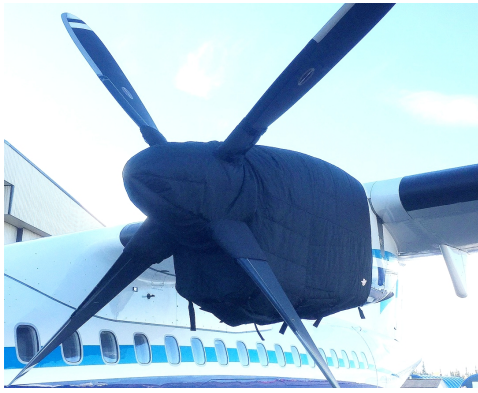
ATR-72-202 Insulated Engine & Prop Hub Covers
