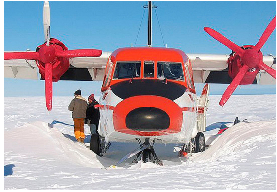
Casa 212 Insulated Engine & Propellor/Spinner Covers
