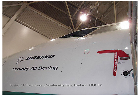
Boeing 737 Heat Resistant Pitot Cover
