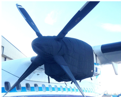
ATR-72-202 Insulated Engine & Prop Hub Covers
