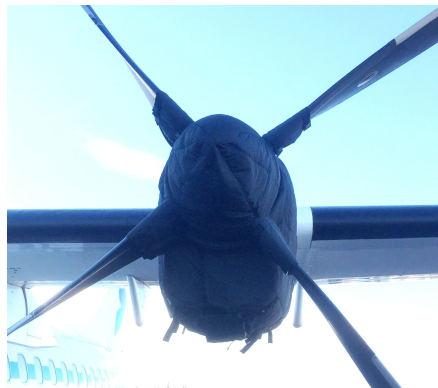
ATR-72-202 Insulated Engine & Prop Hub Covers
