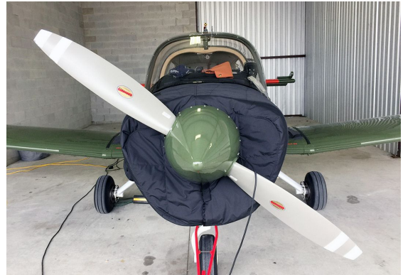
Scottish Aviation Bulldog Insulated Engine Cover
