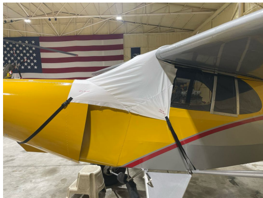
Piper J5A Windshield/Skylight Cover, test fit
