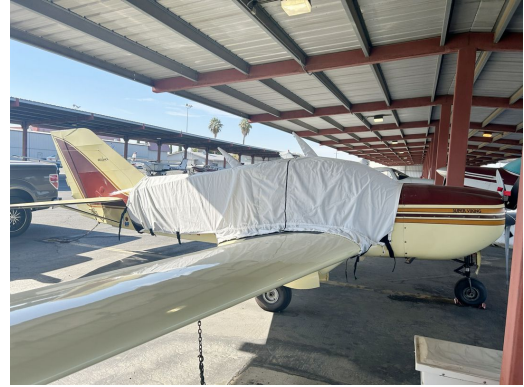
Bellanca Viking Extended Canopy Cover & 12" Wing Extensions (to LE of Horizontal Stabilizer)
