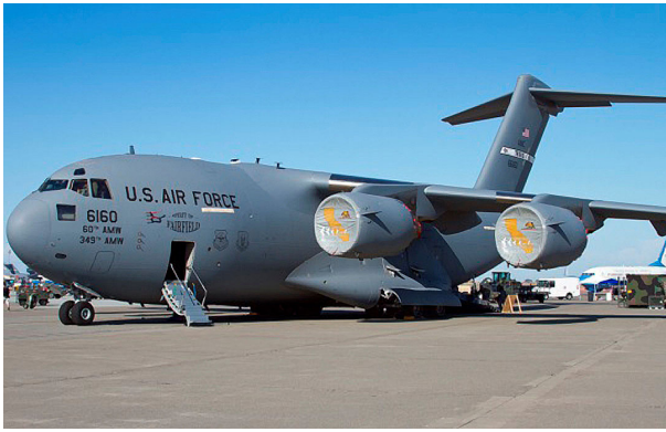
C-17 Engine Intake Covers and Exhaust Covers
