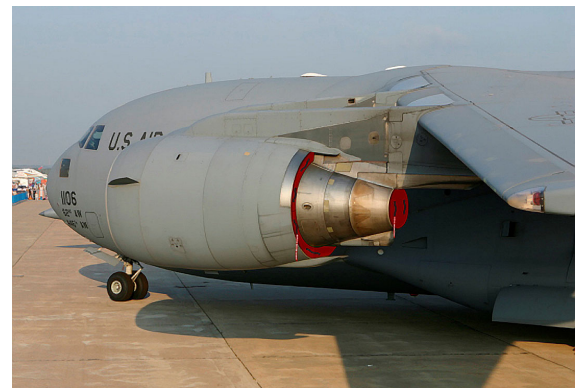
C-17 Bypass and Exhaust Plugs (illustration)
