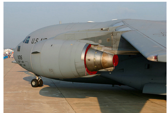
C-17 Bypass and Exhaust Plugs (illustration)
