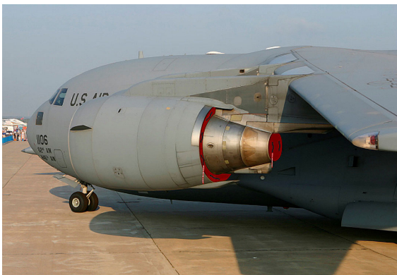
C-17 Bypass and Exhaust Plugs (illustration)
