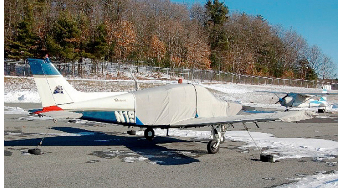
Beech Sierra Prop, Engine, Extended Canopy, Wing, Tailcone, and Horizontal Stab Covers.
