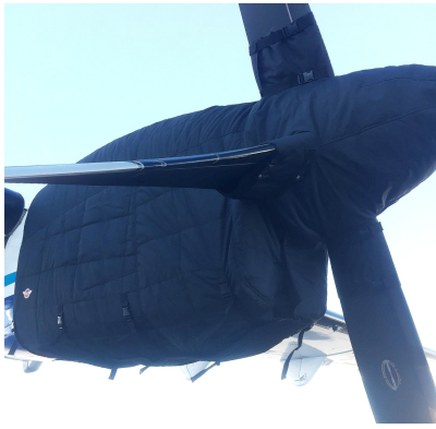
ATR-72-202 Insulated Engine & Prop Hub Covers
