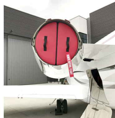
Cessna Citation 680 Exhaust Plugs, folding type
