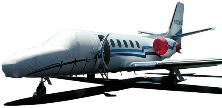
Cessna Citation Nose/Cockpit Cover, Engine Covers
