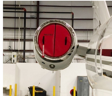
Embraer Legacy 500 Engine Inlet Plugs, folding type
