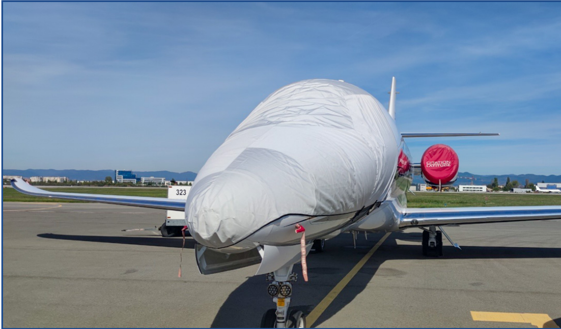
Cessna Citation Latitude (680A) Cockpit/Nose Cover, Doesn't Cover Pitot Tubes
