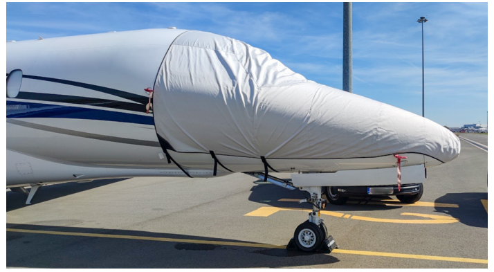
Cessna Citation Latitude (680A) Cockpit/Nose Cover, Doesn't Cover Pitot Tubes
