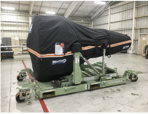
CFM56-5B Off Link Cover, fully enclosed
