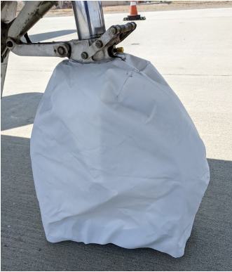
CJ1 Nose Gear Tire Cover, test fit
