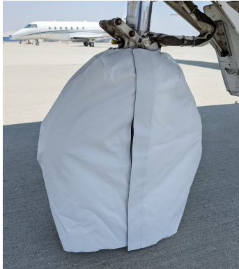
CJ1 Nose Gear Tire Cover, test fit
