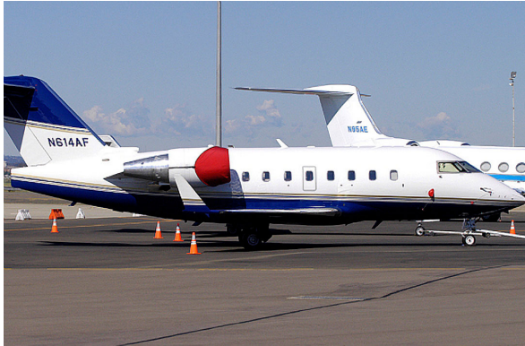
Challenger 604 Intake Covers, standard design
