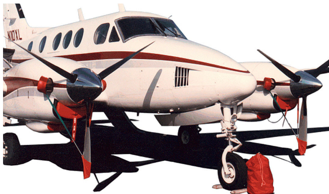
Pitot, Exhaust Covers, Engine Plugs & Prop Ties
