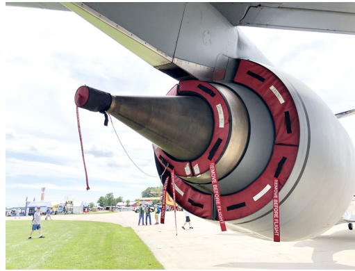
McDonnell Douglas DC-8 Exhaust Plugs, Donut Ring Type For Bypass Vent And Exhaust
