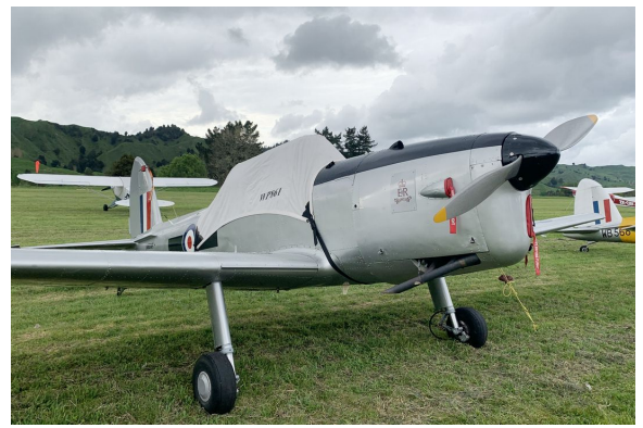
DeHavilland Chipmunk Canopy Cover, Engine Plugs
