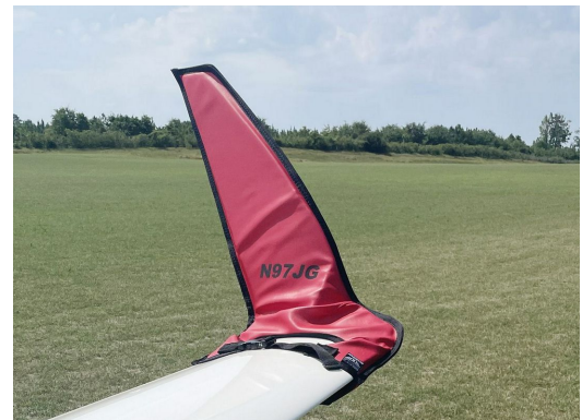
Schempp-Hirth Ventus-2B winglet/wingtip pads
