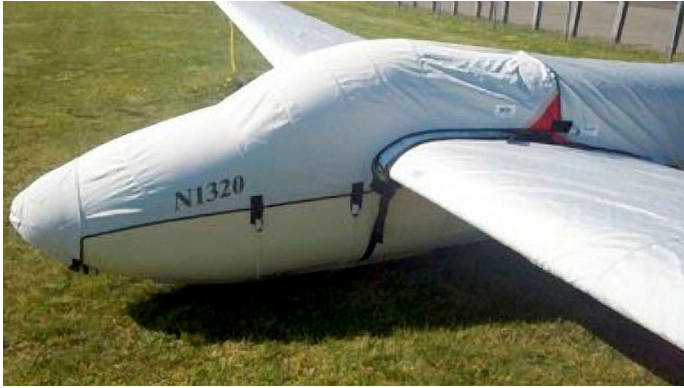
Schweizer SGS 1-26B Canopy/Nose, Wings & Empennage Covers
