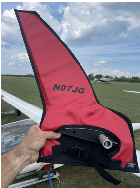
Schempp-Hirth Ventus-2B winglet/wingtip pads
